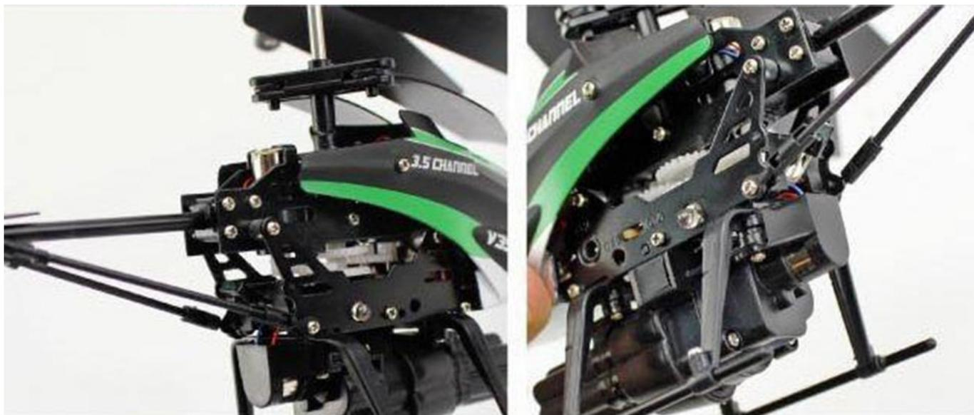
Alloy frame and flexible plastic material, with double motor power system, provide high efficiency power to fly.
